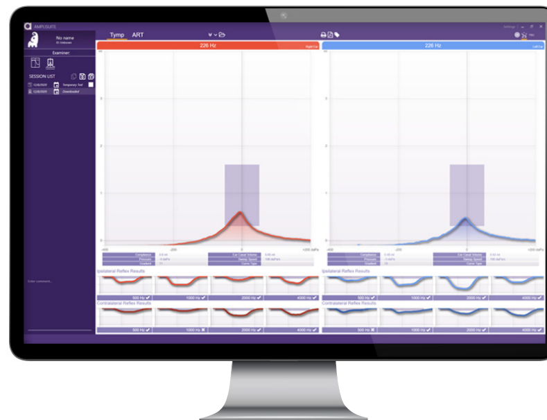
The tympanometry module includes both tympanometry and acoustic reflex graphs
