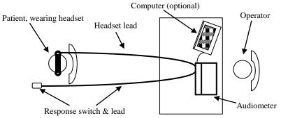
The patient is seated in front of the desk facing away from the operator. The patient wears a headset or appropriate transducer (see Section 4.3) and responds to test stimuli by use of a hand-held switch which is also connected to the instrument.
