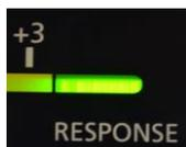
When the test person is pressing the patient response switch, the LED above the display labeled with **RESPONSE** will illuminate.
