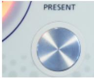
The presentation button is located to the right of the Channel 1 rotary control. The button is conductive, by touching it the test signal will be presented to the patient (presentation mode) or interrupted (continuous mode).
