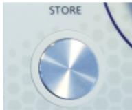
The store button is located to the left of the Channel 2 rotary control. The button is conductive, by touching it the current test level and frequency will be stored to the temporary memory of the device.
