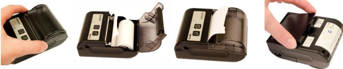
1. Open the lid by pushing on the sides, insert paper roll as shown,
