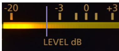
⊘ VU meter does not reach 0dB line
