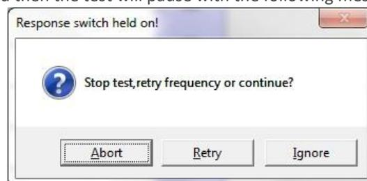
Depending on circumstances the operator may choose to abort the test, retry the frequency, or ignore the error (and proceed to testing of the next frequency).
