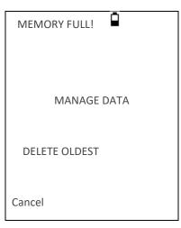
Selecting MANAGE DATA will display the DATA MANAGEMENT menu which provides options for printing or transferring data to a computer prior to deleting records to make space for the new test.
