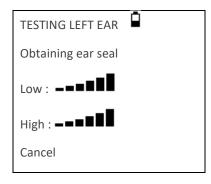
The number of bars shown indicates the robustness of the seal. The probe should be adjusted in the ear until two or more bars are shown for Low & High.
