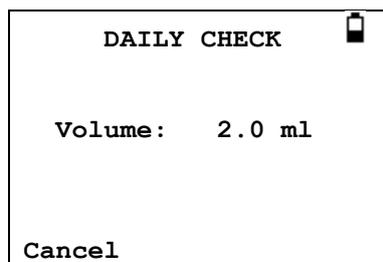
Remove the probe and repeat the test with the three remaining test cavities. The display should show the volume of the 0.2ml, & 0.5ml test cavities to within  $\pm 0.1$ ml. The volume of the 5.0ml test cavity should be shown within  $\pm 0.25$ ml.
