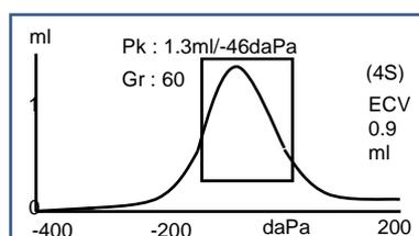
The default display mode is +200daPa offset (as shown in the diagram on the left and indicated by 2S on the display) but an offset of -400daPa may be selected if required (as shown in the diagram on the right and indicated by 4S on the display). See Section 5.5.3 for details of how to switch between the available display modes.
