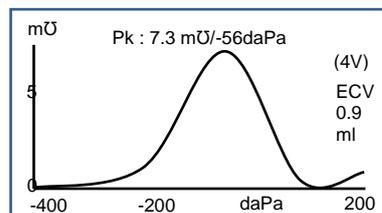
The format is generally similar to that used for scalar mode with the 1000Hz probe tone. Again, the +200daPa offset (2V) and -400daPa offset (4V) are available as required.
