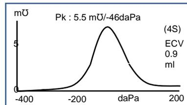
The default 1000Hz display mode is Scalar with -400daPa offset (as shown in the diagram on the right and indicated by 4S on the display) but alternative 1000Hz modes may be selected if required (see Section 5.5.3). The units displayed on the vertical axis are mmho (mU) which is normal practice for 1000Hz operation. The ear canal volume (ECV) is shown in ml.
