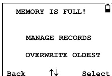
Selecting MANAGE RECORDS will display the DATA MANAGEMENT menu (Section 9) which provides options for printing or transferring data to a computer prior to deleting records to make space for the new test.
