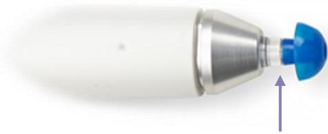
Ensure that the ear tip is pushed all the way down on the probe tip and that there is no gap between probe tip and ear tip.
