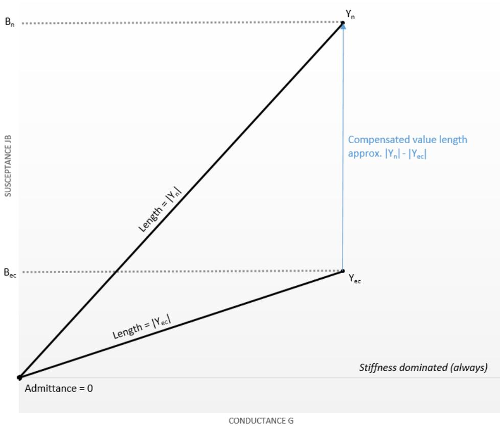
**Figure 1:** 226 Hz probe tone: The distance between the  $n^{\text{th}}$  sample  $Y_n$  (admittance value of the  $n^{\text{th}}$  sample in the tympanogram) and the baseline sample  $Y_{ec}$  is essentially the same as the difference in lengths between the length  $|Y_{ec}|$  because conductance is always small at 226 Hz and reading are always stiffness dominated. Scalar subtraction  $(|Y_n| - |Y_{ec}|)$  is adequate.
