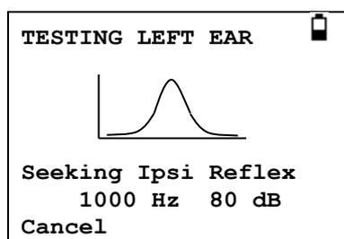
The display changes to show the frequency and level being used, starting with the lowest frequency and level selected.
