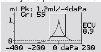
To record the tympanogram, the admittance is measured while the air pressure in the ear canal is varied from +200 daPa to -400 daPa by means of a small pump. The admittance peaks when the air pressure is the same on both sides of the tympanic membrane. The change of admittance with pressure is displayed graphically.
