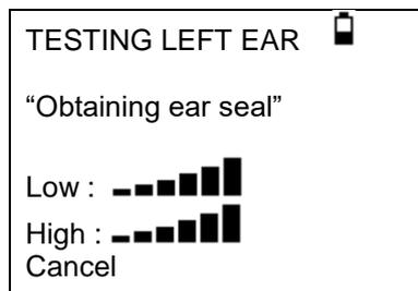
The number of bars shown indicates the robustness of the seal. The probe should be adjusted in the ear until two or more bars are shown for Low & High. The method used for the thorough ear seal check places a maximum limit on the ear canal volume of ~4.5ml.
