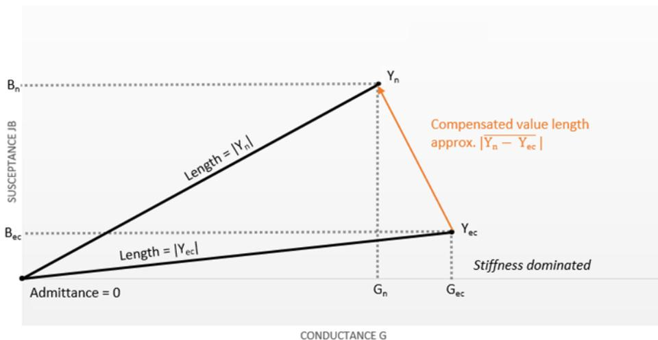
**Figure 2:** 1 kHz probe tone: Although the susceptance values  $B_n$  and  $B_{ec}$  are the same as in the 226 Hz diagram, the distance between the  $n^{\text{th}}$  sample  $Y_n$  and the baseline sample  $Y_{ec}$  is nothing like the difference in lengths between  $Y_n$  and  $Y_{ec}$  (which here would be close to 0), due to the conductance values and the possibility of mass dominated measurements. Vector subtraction  $(\overline{Y_n} - \overline{Y_{ec}})$  is necessary.
