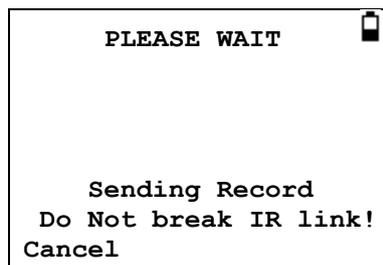
If a connection cannot be made the print operation will time out (Able AP1300 printer only – after approximately 30sec) and the following message will be displayed. The same message will occur if the print operation is cancelled at this stage.
