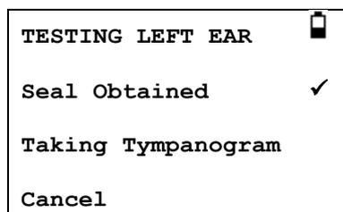
Once an adequate seal is detected the tympanogram measurement is made. This takes about 3 seconds. It is important not to move the probe and to ask the patient to remain very still during the test.
