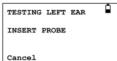
Present the ear tip to the ear and obtain a seal. If a good seal has been detected the following sequence of messages will be seen
