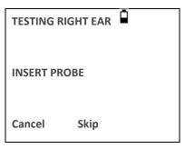
Press ► to skip testing of the right ear and display the PROCESS RESULTS menu. Press ◀ to cancel and return to the ear selection menu. In both cases the left ear results are retained and may be viewed as the LAST TEST.
