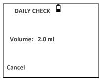
Remove the probe and repeat the test with the three remaining test cavities. The display should show the volume of the 0.2ml, & 0.5ml test cavities to within  $\pm$  0.1ml. The volume of the 5.0ml test cavity should be shown within  $\pm$  0.25ml.
