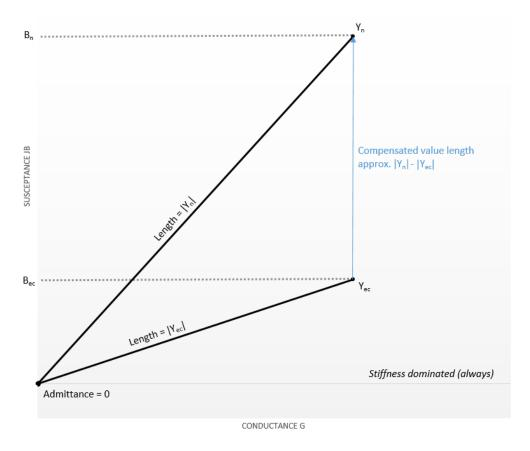
$\textbf{Figure 1:}\ 226\ \text{Hz probe tone:}\ \text{The distance between the }n^{th}\ \text{sample }Y_n\ (\text{admittance value of the }n^{th}\ \text{sample in the tympanogram})\ \text{and}$ the baseline sample  $Y_{ec}$  is essentially the same as the difference in lengths between the length  $|Y\_{ec}|$  because conductance is always small at 226 Hz and reading are always stiffness dominated. Scalar subtraction ( $|Y_n| - |Y_ec|$ ) is adequate.
