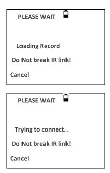
The Otowave 202 will then attempt to connect to the printer. When this has been done the data will be transferred. During this time the following message is displayed.
