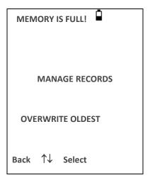
Selecting MANAGE RECORDS will display the DATA MANAGEMENT menu (Section 9) which provides options for printing or transferring data to a computer prior to deleting records to make space for the new test.
