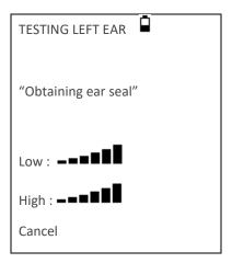
The number of bars shown indicates the robustness of the seal. The probe should be adjusted in the ear until two or more bars are shown for Low & High. The method used for the thorough ear seal check places a maximum limit on the ear canal volume of ~4.5ml.
