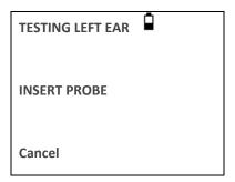
Present the ear tip to the ear and obtain a seal. If a good seal has been detected the following sequence of messages will be seen
