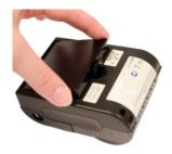
Open the lid by pushing on the sides, insert paper roll as shown, and close the lid.
