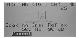
The acoustic reflex test screen consists of the preview of the measured tympanogram. Underneath the graph, the tested ear, the test frequency and intensity are listed. The reflex test starts with the lowest frequency and level selected.
