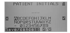
To enter the data, use the ▲ ▼ ◀ and ▶ keys to select a character. Press and hold the ▶ key to enter the selected character. To delete the last character, press and hold the ◀ key.
