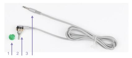
1 Ear tip Ear tip to be placed on probe tip of contra phone
