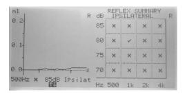
If Reflex autostop has not been selected the larger scale trace of the reflex at the lowest frequency with the lowest level that gave a response is shown on the left hand side of the screen.
