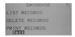
Up to 36 tests can be stored in the Otowave 302+ internal database.
