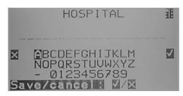
To enter the data use the  $\blacktriangle$   $\blacktriangledown$   $\blacktriangleleft$  and  $\blacktriangleright$  keys to select a character. Press and hold the  $\blacktriangleright$  key to enter the selected character. To delete the last character, press and hold the  $\blacktriangleleft$  key.
