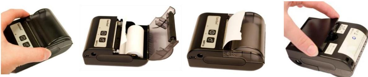
1. Open the lid by pushing on the sides, insert paper roll as shown, and close the lid.
