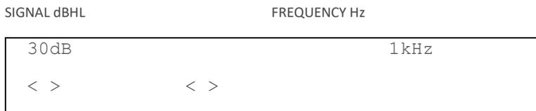
This indicates that the audiometer is now ready to be used for automatic testing which is initiated by Audibase and controlled by the PC850 software.
