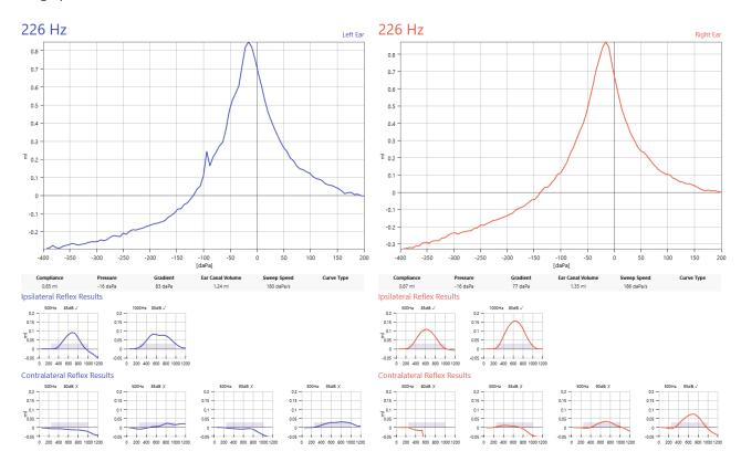
On the tympanometry graphs, the option is given to show a normative box. This area is intended to help identify normal tymp curves, according to default or customised specifications. In the case that the peak of the curve falls into the normative area, the tymp is marked with a  $\checkmark$  to identify a normal shaped curve.
