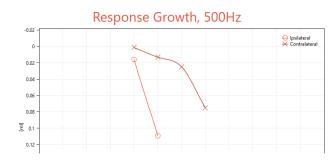
The acoustic reflex magnitude increases as the stimulus level increases. The peak magnitude of the reflex is plotted for each level tested, resulting in a reflex growth function.
