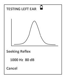
The display changes to show the frequency and level being used, starting with the lowest frequency and level selected.
