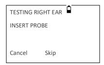
Press ► to skip testing of the right ear and display the PROCESS RESULTS menu. Press ◀ to cancel and return to the ear selection menu. In both cases the left ear results are retained and may be viewed as the LAST TEST.
