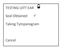
Once an adequate seal is detected the tympanogram measurement is made. This takes about 3 seconds. It is important not to move the probe and to ask the patient to remain very still during the test.
