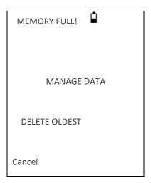
Selecting MANAGE DATA will display the DATA MANAGEMENT menu which provides options for printing or transferring data to a computer prior to deleting records to make space for the new test.
