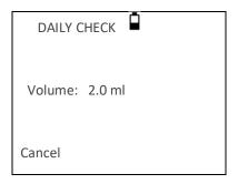
Remove the probe and repeat the test with the three remaining test cavities. The display should show the volume of the 0.2ml and 0.5ml test cavities to within ± 0.1ml. The 5.0ml test cavity should be within ± 0.25ml.
