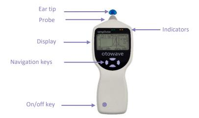
The indicators show the status of the system. Typical indications during a measurement sequence are as follows:
