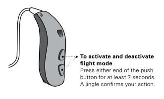
Opening and closing the battery drawer will deactivate the flight mode. See section "Quick reset".
