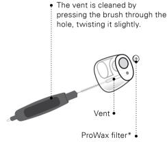
\* VarioTherm<sup>®</sup> Micro Mold and Lite Tip do not have a wax filter.
