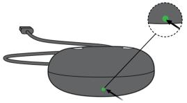
When the charger is connected to power, the green LED turns on.
