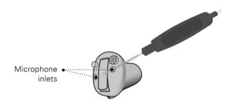
Clean the vent by pressing the brush through the hole while twisting it slightly.
