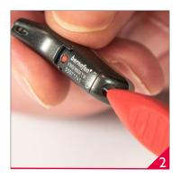
Insert the service tool at an angle as shown in the battery drawer release hole to open the battery drawer.
