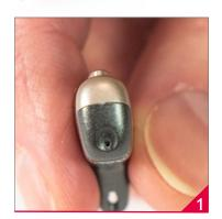
Look for the battery drawer release hole on the bottom of the instrument.
