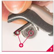
Use gloves to place the new battery as shown with the + sign facing up for both the battery and the battery drawer.
