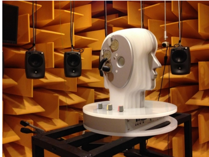
Figure 2: The Klangfinder HS8 Pro artificial head wearing all three devices.
