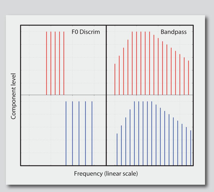
Fig.2. Representation of test stimuli. The left column shows stimuli used for a FO discrimination task. The right column shows harmonic and frequency shifted tones which have a similar envelope repetition rate but different TFS
