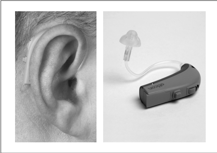
Figure 6.3. 'Thin-Tube Open Fitting' hearing aid: to the left, placed in the ear; to the right, placed on a table so that all the outer parts of the hearing aid are visible, including the thin tubing and the open ear mold
