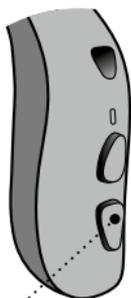
To activate and deactivate flight mode press and hold the Program Button (lower part) for 7 seconds.
