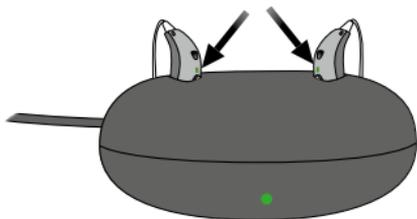
The LEDs on the hearing aids will turn on when the hearing aids are correctly placed in the charger.
