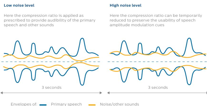
**Figure 2:** Envelopes of speech and noise at two different noise levels; low (left) and high (right)
