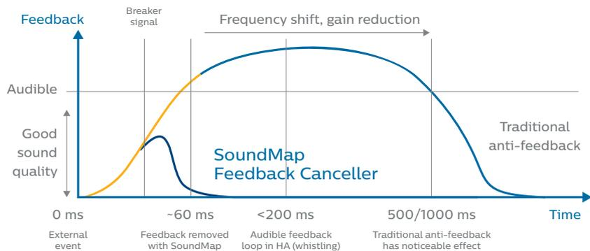
**Figure 6:** Growth and management of feedback in hearing aids. After an abrupt initial acoustical change around the hearing aid (e.g. phone to the ear), a feedback loop can be triggered, and feedback whistling may become audible. The figure shows the difference in reaction time between a traditional anti-feedback strategy, which often reacts after feedback has become audible and SoundMap Feedback Cancellor, which can prevent feedback while it is still building up and not yet audible.
