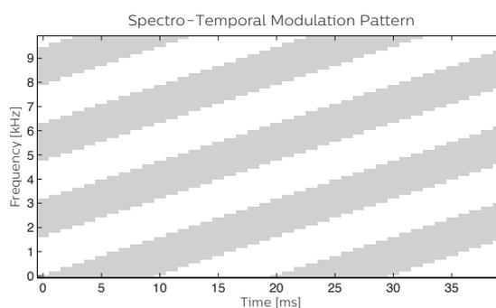
**Figure 7:** Illustration of the breaker signal used in SoundMap Feedback Cancellation
