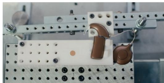
Sound processor battery compartment test – 6,000 cycles
