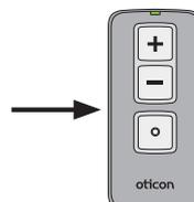
Briefly press any key on the remote control to make it automatically pair with the instrument(s).
