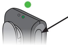
Press and hold the multibutton for approx. 3 sec. until power indicator STEADY Green ●
