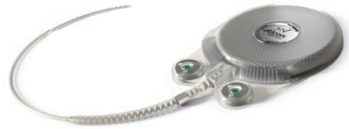
Figure 2: Neuro Zti with the new magnet
