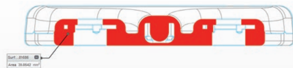
Figure 6: Cross section of Neuro Zti implant showing the higher mechanical resistance areas in red
