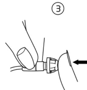
Under the dome you will notice a white wax filter attached to the end of the speaker. This is a wax filter that will keep debris from damaging the speaker. If this filter becomes clogged, contact your Hearing Care Professional for service and replacement of the filter.
