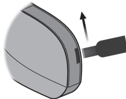
Insert the screwdriver into the slit on the back of the hearing aid. Close the drawer using your fingers. Make sure the drawer is completely closed.
