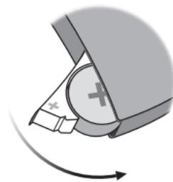
Close the battery drawer. The hearing aid will play a jingle through the earpiece. Hold the earpiece close to your ear to hear the jingle.
