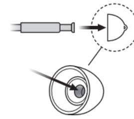
Insert the thin tube exactly into the middle of the earpiece to obtain a secure attachment.
