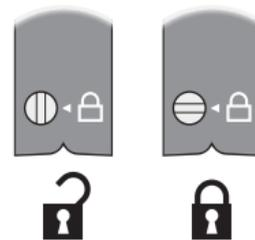
Make sure the drawer is completely closed. Turn the screw to the locked position (horizontal).
