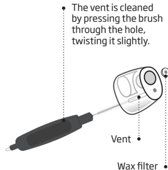
• The vent is cleaned by pressing the brush through the hole, twisting it slightly.
