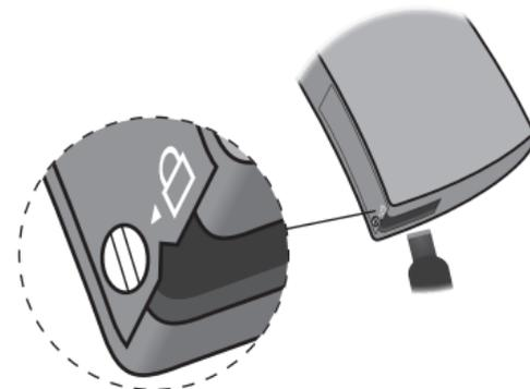
Use the screwdriver to turn the screw to unlock position (vertical). Insert the screwdriver into the slit in the bottom of the hearing aid and push the door open.
