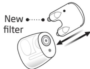
Push the empty pin into the wax filter in the earpiece and pull it out.
