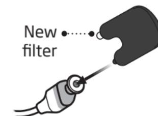
Push the empty pin into the wax filter in the speaker and pull it out.
