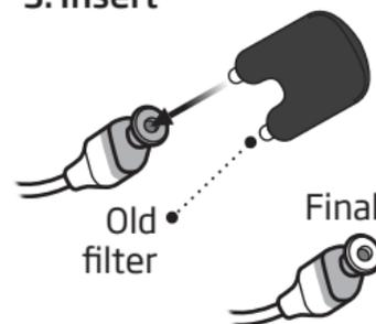
Insert the new wax filter using the other pin, remove the tool and throw it out.
