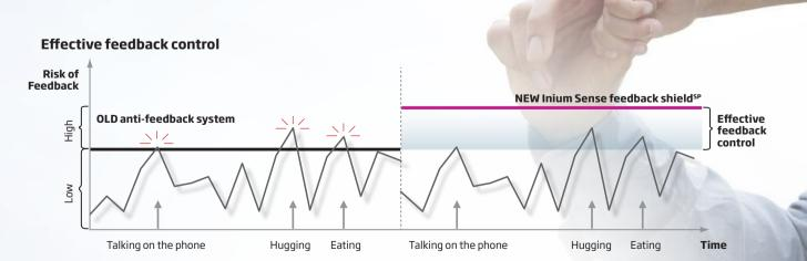
Inium Sense feedback shield<sup>SP</sup> lifts Dynamo out of the area of feedback risk by effective feedback control. When critical acoustic events occur as part of a typical day, effective feedback control ensures continuously high sound quality by eliminating feedback efficiently.
