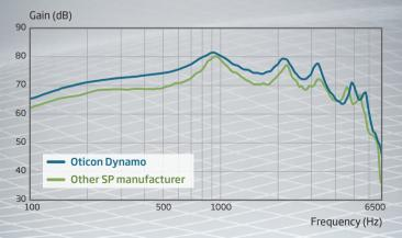
Full-On Gain measurements performed in technical settings according to IEC-60118 (711 coupler). Oticon Dynamo (blue) and other manufacturer (green). Both super power devices are size 13 battery.
