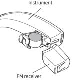
If you would like to receive input from the FM transmitter alone, you can switch forwards to the next FM programme by using the programme switch button.
