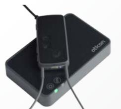
Place the Streamer on top of the phone adapter - the pairing takes around 20-60 seconds. The pairing is completed when the power indicator on the phone adapter and the on/off indicator on the Streamer turns steady blue.
