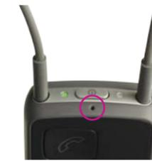
Wear the Streamer around the neck and make sure not to cover the microphone with clothes. Make sure that you are able to speak into the Streamer's microphone inlet.
