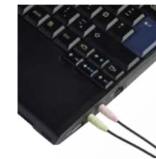
Plug the splitter cable in the computers microphone input (pink)/audio output (green).
