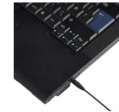
Plug the mini jack stereo cable in the computer.
