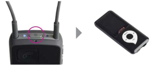
Bring Streamer in pairing mode by pressing the on/off button on top of the Streamer Pro for five seconds until the blue light starts blinking.
