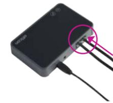
Plug the "phone cable" (Included in the phone adapter package) in the phone adapter "OUT" connector.
