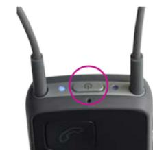
Bring Streamer in pairing mode by pressing the on/off button on top of the Streamer for 5-6 seconds until the blue light starts blinking.
