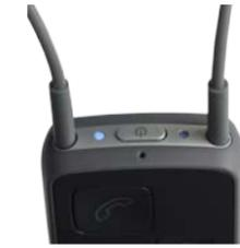
Bring the Streamer in pairing mode by pressing the on/off button on top of the Streamer for five seconds until the blue light starts blinking.
