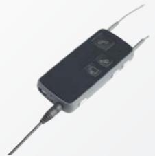
Plug in the mini jack stereo cable to the Streamer's input/output mini jack at the bottom of the Streamer.
