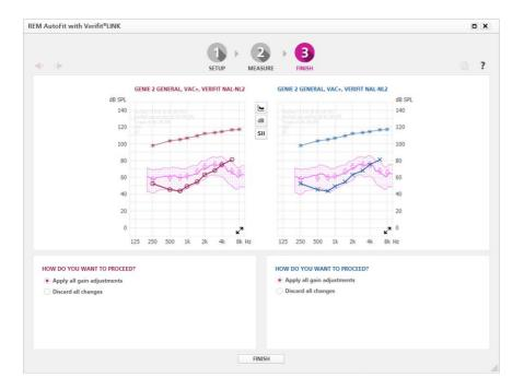
The graph now displays the instrument output most recently measured in your client's ear or in the test-box, and you can apply the adjustments from the Measure step. The graphs and instruments will update according to what you select:
