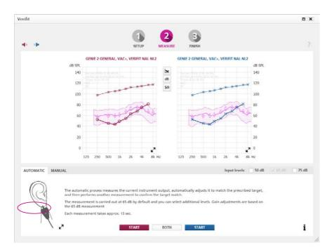
**Automatic**: measures the current instrument output, automatically adjusts it to match the prescribed target, and then performs another measurement to confirm the target match.
