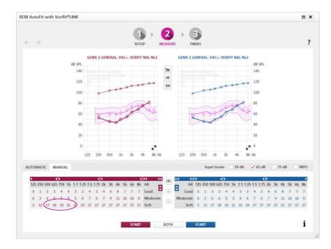
**Manual**: lets you fine-tune the instrument gain to get even closer to target or to personalise the fitting based on your client's comments. This manual process can be done after or instead of the automatic process. Within the REM AutoFit tool, use the fine-tuning controls to adjust the gain and then manually run a measurement to verify the target match.
