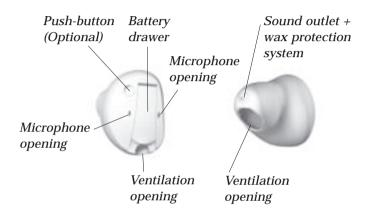
Battery size: 10 (without push-button) Battery size: 312 (with push-button)
