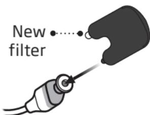
Push the empty pin into the wax filter in the speaker and pull it out.
