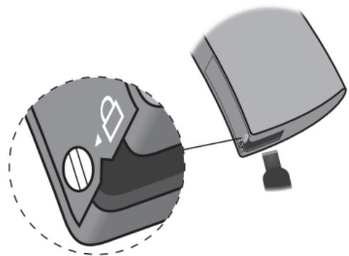
Use the screwdriver to turn the screw to unlock position (vertical). Insert the screwdriver into the slit in the bottom of the hearing aid and push the drawer open.
