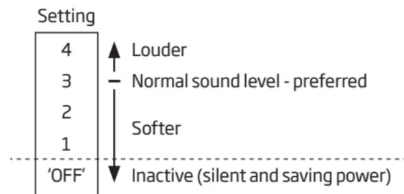
The normal volume wheel setting is 3. When adjusting the volume to the normal level you will hear a double beep.
