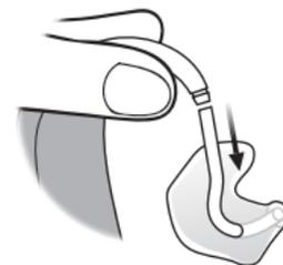
Disconnect the tube and mould from the hook. Hold the hook firmly, when pulling off the tube. Otherwise the hearing aid may be damaged.
