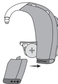
Start by opening the battery door and slide the DAI adapter onto the hearing aid.
