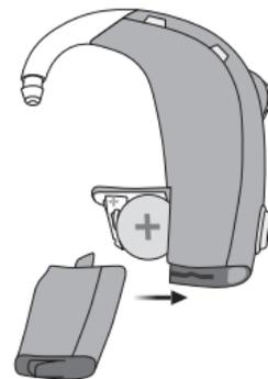
Start by opening the battery door. Slide the FM receiver onto the hearing aid.
