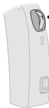
Use the volume wheel to mute the hearing aid by turning below setting 1 until it clicks. To reactivate the hearing aid, turn up on the volume wheel.
