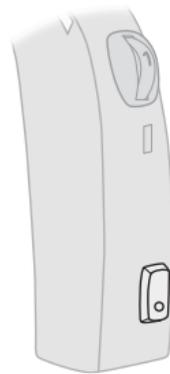
Apply a very long press to the button to mute the hearing aid. To reactivate the hearing aid, push the button briefly.
