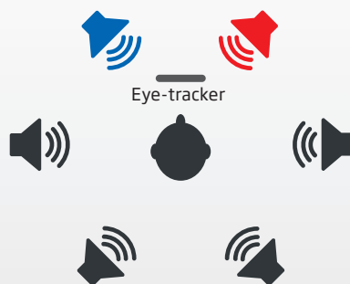
Figure 1. Test setup with a total of six loudspeakers, which is identical to the setup used in the Oticon More EEG study (Santurette et al., 2020). Pupillometry was done by placing an eye-tracker in front of the participants to measure sustained listening effort. Two frontal loudspeakers (blue and red) contained a male and a female talker reading audio clips simultaneously. Background noise, which is a 16-talker babble, came from the remaining four loudspeakers.
