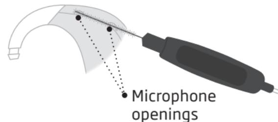
Make sure that no parts of the MultiTool are squeezed into the microphone openings by force. This may damage the hearing aid.
