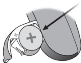
Insert the new battery into the battery drawer. Make sure the + side is facing up.
