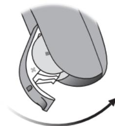
Close the battery door completely and make sure it is locked.
