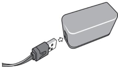
Plug the USB into the charger, then plug the adapter into the wall. Once powered, the charger LED will shortly blink green.
