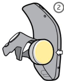
2. Place the ZPower rechargeable battery inside the battery drawer (gold side facing upwards)
