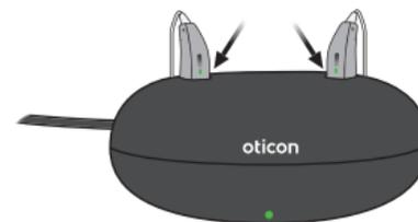
The hearing aids LEDs will turn on when the hearing aids are correctly placed in the charger.
