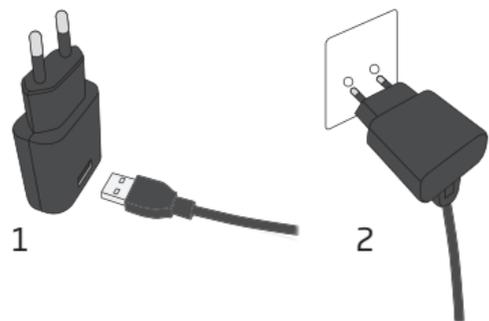
1. Insert the USB plug into the power plug.
