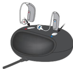
Place the hearing aids in the charging ports as shown in the picture. Make sure that the hearing aids match the right and left indicators on the charger.
