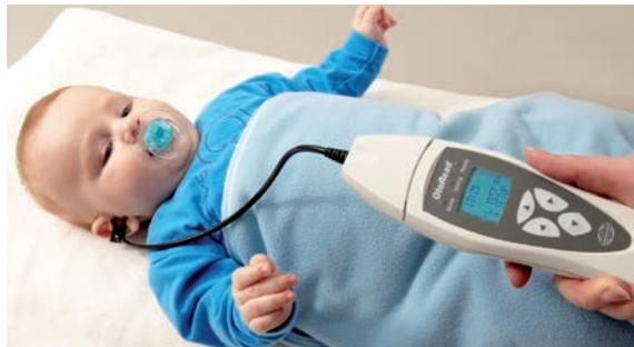
*An OAE screening with Interacoustics Otoread. OAE testing is characterized by fast test time, low consumable costs and a relatively higher number of referrals for diagnostic follow-up.*
