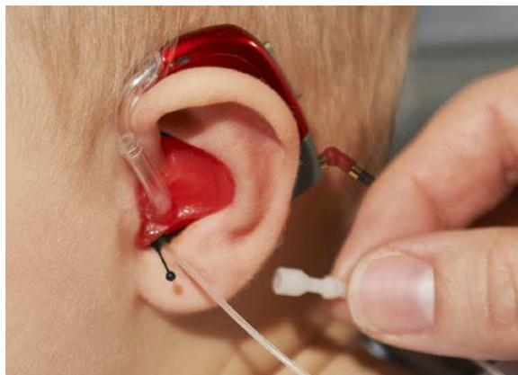
*Hearing aid with programming cable attached and Real Ear Measurement insitu tube.*
