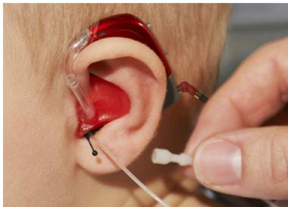
*Hearing aid with programming cable attached and Real Ear Measurement insitu tube.*
