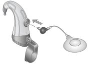
6 Rotate the plug 90 degrees clockwise to lock it in place.
