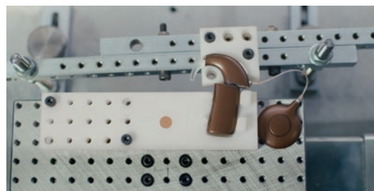
Sound processor battery compartment test – 6,000 cycles
