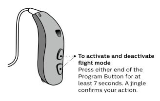
Opening and closing the battery drawer will deactivate the flight mode. See section "Quick reset".
