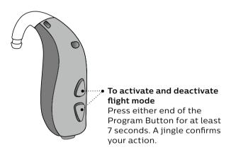
Opening and closing the battery drawer will deactivate the flight mode. See section "Quick reset".
