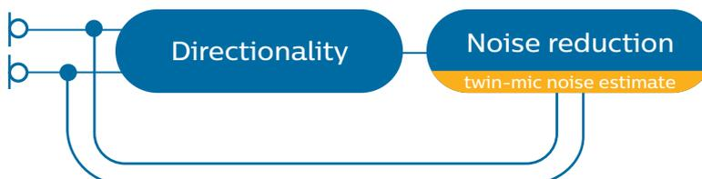
Figure 4: SoundMap Noise Control with its twin-microphone noise estimate
