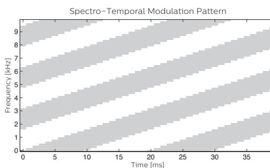
**Figure 7:** Illustration of the breaker signal used in SoundMap Feedback Cancellation
