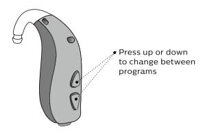
You can change continuously between programs both up and down in the program order. For example, if you want to go from program 1 to 4, you can press the down button once instead of pressing the up button 3 times.
