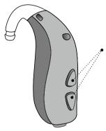
Apply a very long press (4 seconds) to either end of the Program Button to mute the hearing aid.
